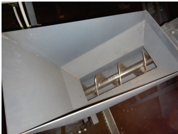
Fig. 8. Access to the entanglement and crushing zone in the binder charging hopper
