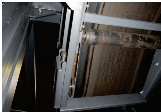
Fig. 7. Access to the catching area between support roller and belt and between the belt and reversable roller
