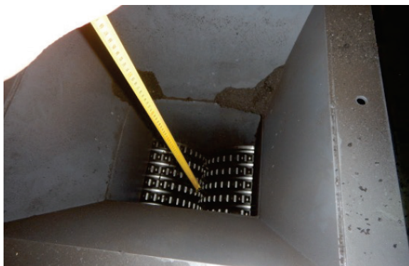
Fig. 9. Access to the catching and crushing zone of the briquetting press
