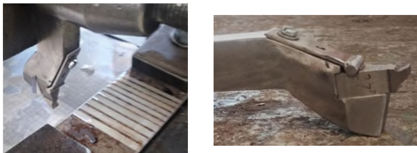
Fig. 5. Planer tool as a physical model of broaching process
