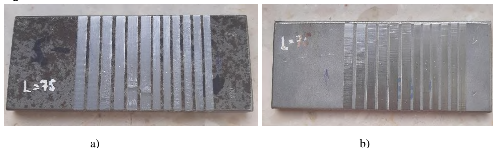
Fig. 6. Photos of samples after machining from grade steel: a) 1.7335 (13CrMo4-5, 15HM); b) 1.4841 (X15CrNiSi25-21, H25N20S2)
