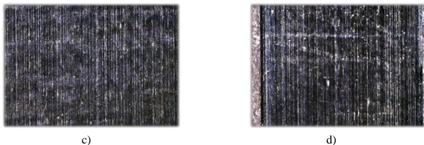
Fig. 9. Photo of the machining grooves surface magnification \times 36 : a) Ra_{avg} = 1.02 \mu\text{m} (steel 1.4841, test number 6); b) Ra_{avg} = 12.85 \mu\text{m} (steel 1.4841, test number 10); c) Ra_{avg} = 0.52 \mu\text{m} (steel 1.7335, test number 6); d) Ra_{avg} = 1.79 \mu\text{m} (steel 1.7335, test number 1)
