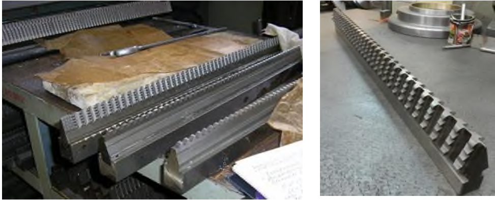
Fig. 4. Broaches used to machining turbine disk lock groove
