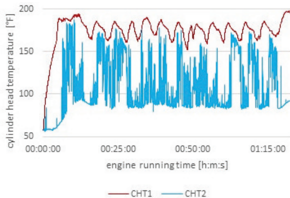
Fig. 5. Cylinder head temperature indications with one faulty sensor [4]
